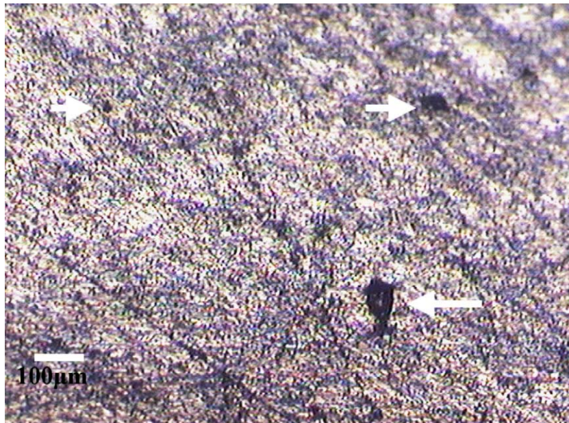
Fig. 8. Optical microphotograph of composite bipolar plate with 80 wt.% graphite content ( \times 50 ).
